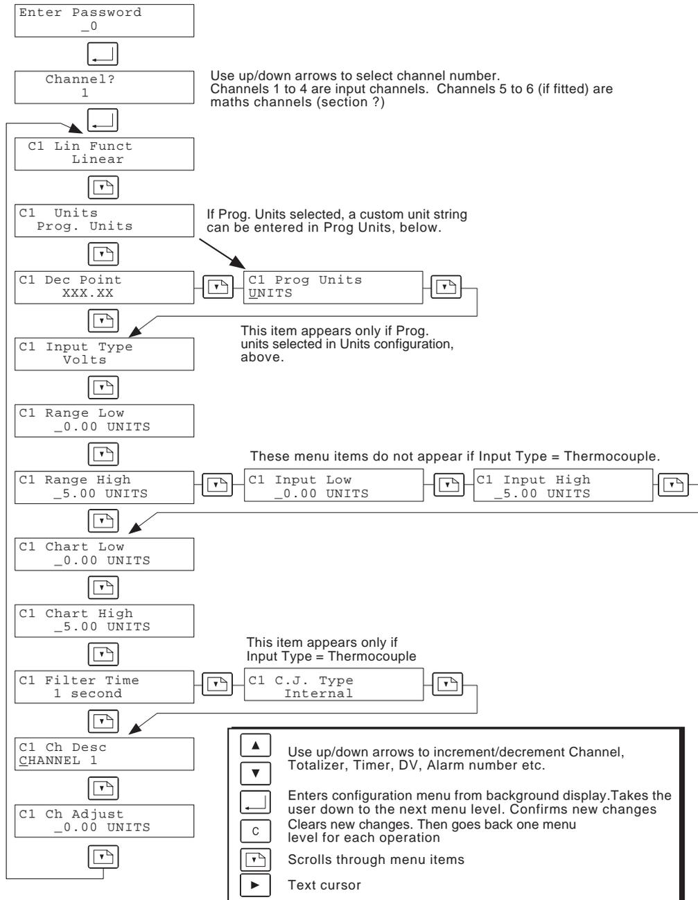
Figure 4.3 Input channel configuration menu structure
