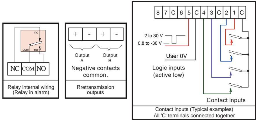
Figure 2.2.3b Option wiring
