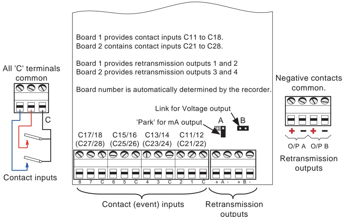
Figure 4.11.1 Retransmission/contact input: Hardware configuration and pinout
