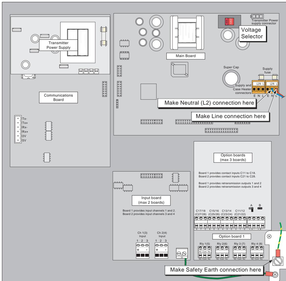
Figure 2.2.1 Circuit board location, and Supply Voltage connection
