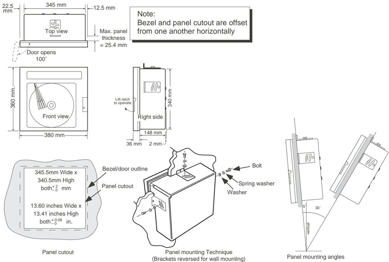
Figure 2.1 Mechanical installation
