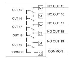
Fig. 11.C RELAY OUTPUTS 15 to 19 WIRING
