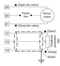
Fig. 15 SERVOMOTOR OUTPUT WIRING
