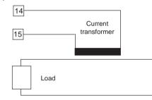
Fig. 10 CURRENT TRANSFORMER INPUT WIRING This input allows you to measure and display the current running in the load, driven by a time proportional control output, during the ON and OFF periods of the output cycle time. By this feature it is also available the "Output failure detection" function (see page 110).
