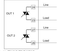
Fig. 14 TRIAC OUTPUT WIRING
