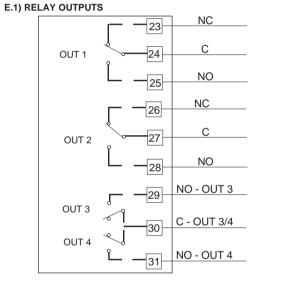
Fig. 11.A RELAY OUTPUTS 1,2,3 and 4 WIRING
