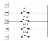
Fig. 9.B - LOGIC INPUTS IN 1, 2, 3 and 4 WIRING
