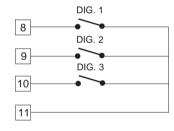
Fig. 9.A - LOGIC INPUTS DIG 1, 2, 3 WIRING
