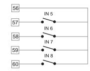
Fig. 9.C - LOGIC INPUTS IN 5, 6, 7 and 8 WIRING
