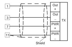
Fig. 7.C INPUTS WIRING FOR 4-WIRE TRANSMITTER
