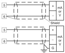
Fig. 8 AUXILIARY INPUT WIRING
