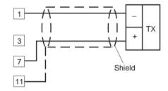
Fig. 7.A INPUTS WIRING FOR 2-WIRE TRANSMITTER
