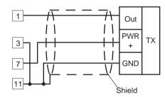
Fig. 7.B INPUTS WIRING FOR 3-WIRE TRANSMITTER
