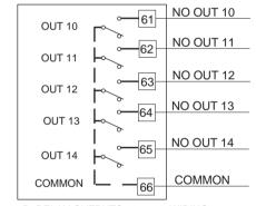
Fig. 11.B RELAY OUTPUTS 10 to 14 WIRING
