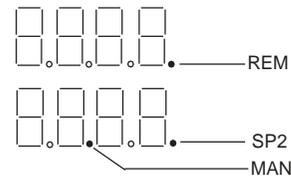
REM = Flashing, when the instrument is controlled via serial link.
